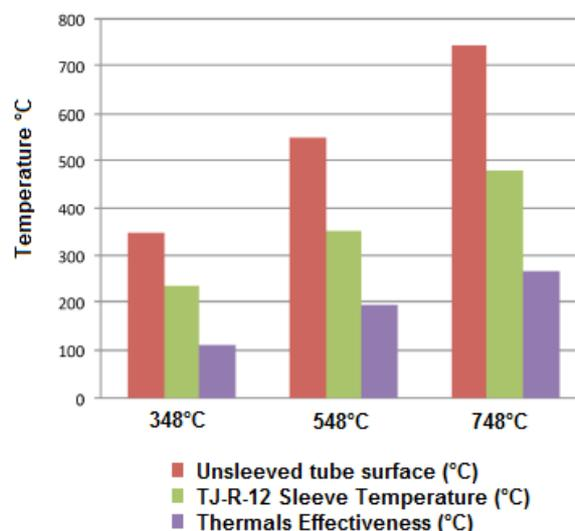
**Note: Thermal effectiveness is the difference between the unsleeved and sleeved tube surface temperatures**
